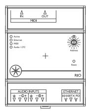
The RIO allows for up to 30 bands of spectrum analysis, so light organ or bar graph type effects can be created using multiple light points. Audio can also be used to manipulate a timeline onto which lighting and video-based effects have been dropped. In this way the time line will move backwards and forwards moving the position of the effects to the music.
