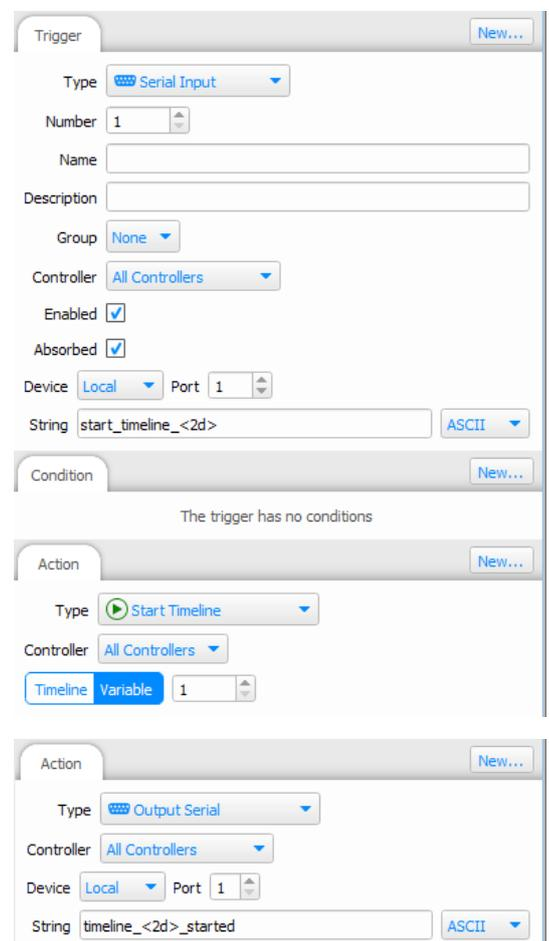
The screenshot displays the configuration interface for a serial trigger and its associated actions. It is divided into three main sections: Trigger, Condition, and Action.
