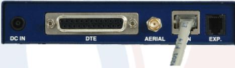
Connect the Ethernet cable to the port labelled "LAN" or "LAN 0" on the rear of the Sarian. The other end of the Ethernet cable must be plugged into a hub or switch to which your PC is also connected.
