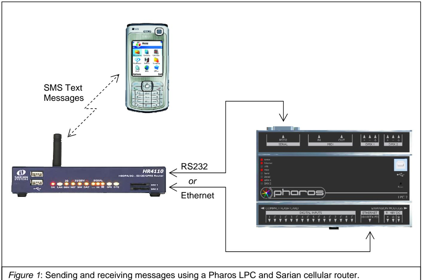
Figure 1: Sending and receiving messages using a Pharos LPC and Sarian cellular router.
