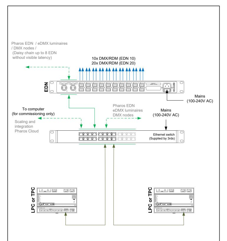
The EDN and controllers need to be in the same project. From there, it is possible to define, per port, which port a controller will output through.
